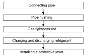
Pipe flushing should be performed once the brazed connections have been completed with the exception of the final connections to the indoor units. That is, flushing should be performed once the outdoor units have been connected but before the indoor units are connected
