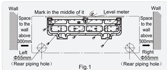
(2) Open a piping hole with the diameter of  $\Phi 55\text{mm}$  on the selected outlet pipe position. In order to drain smoothly, slant the piping hole on the wall slightly downward to the outdoor side with the gradient of  $5-10^\circ$ . (As show in Fig.2)
