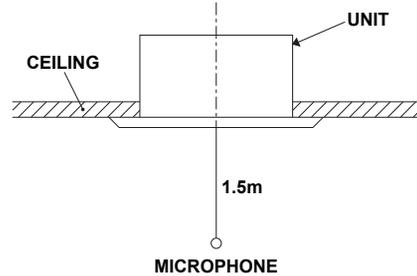
**NOTE:** The sound level is measured in an anechoic room where echoes are few, when compressor stops. The sound may be bigger than the indicated level in actual use due to surrounding echoes. The sound level can be higher by about 2 dB than the indicated level during cooling and heating operation.
